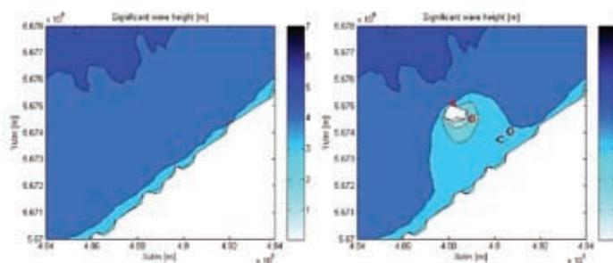
Figure 3: Significant wave height 1000-year storm, NNW direction, (left) without the island, (right) with the island.
