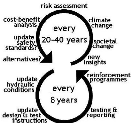
Figure 4: Short term testing and improving flood defences and long-term adjustment to change
