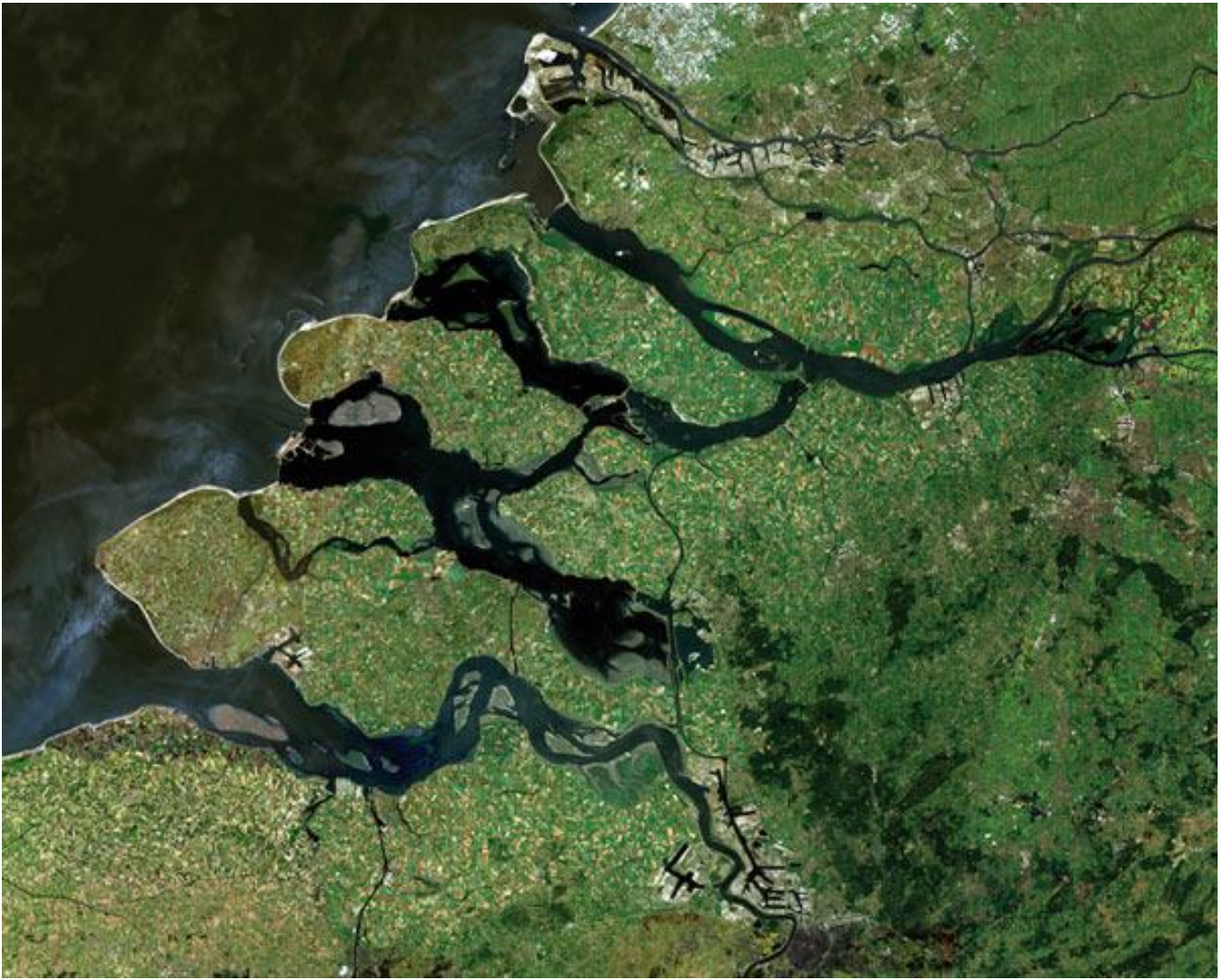
Figure 7: The Delta Project in SW Netherlands between the harbour areas of Rotterdam and Antwerp: the primary dams, sluice complex and storm surge barrier in the west - in the three mouths and three series of compartment dams in the east. (photo: //beeldbank.rws.nl, Rijkswaterstaat)
