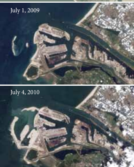
Maasvlakte -2: 2000 ha landreclamation in progress. (photos: NASA)
