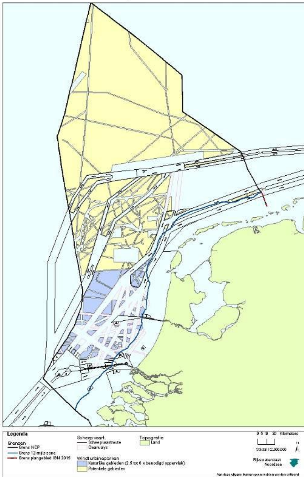
Figure 2: Opportunity map wind farms - blue: favourable areas, yellow: potential areas (source: Policy Document on the North Sea (background document to National Water plan) 2009-2015, December 2009, adapted)
