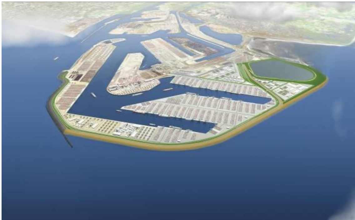
Figure 1: Artistic view of the extension of Rotterdam Harbour, Maasvlakte -2: 2000 ha land reclamation, 2008 - 2013. (source: Rotterdam Port Authority)
