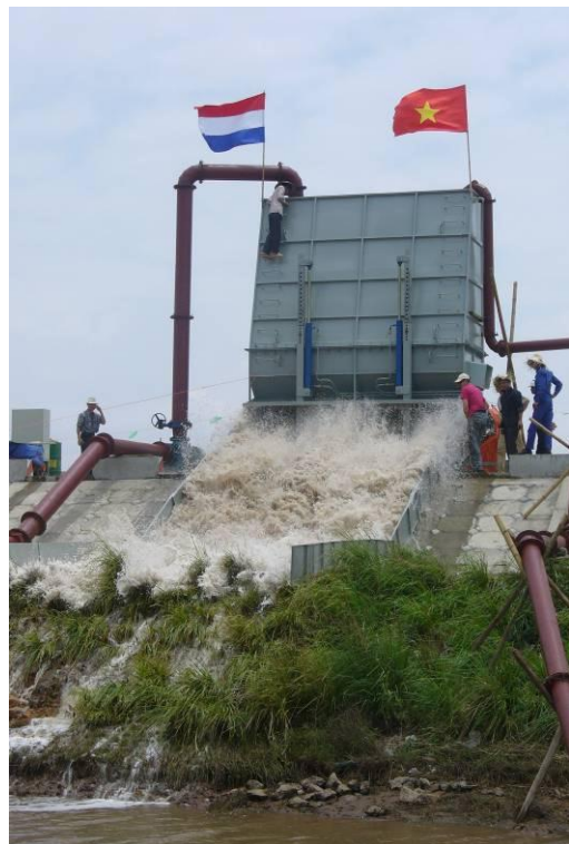
The strength of inner slopes cannot be tested on a small scale and tests have to be done on real dikes. Realistic overtopping volumes are simulated with a Wave Overtopping Simulator in Vietnam on the sea dike in Do Son – Hai Phong, in the same way as is done in the Netherlands. (photo: G.J.Schiereck)
