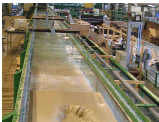
Figure 2: Study on the mechanism sand dune breaching, in the laboratory. (photo: WRU - CE)
