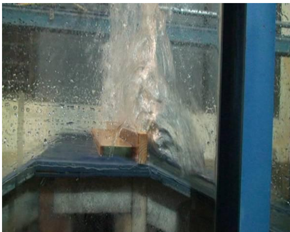
In the wave flume in the hydraulic laboratory of WRU, overtopping tests are undertaken to study e.g. the influence of a crown wall (see wave flume photo above) on overtopping discharges. (photo: H.J. Verhagen)
