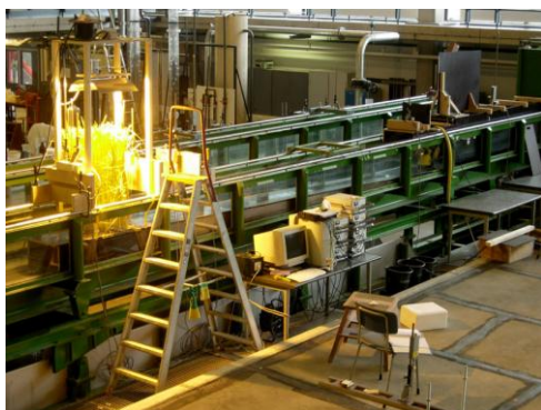
Wave flume testing the reduction of wave overtopping by Vetiver grass. (photo: H.J. Verhagen)
