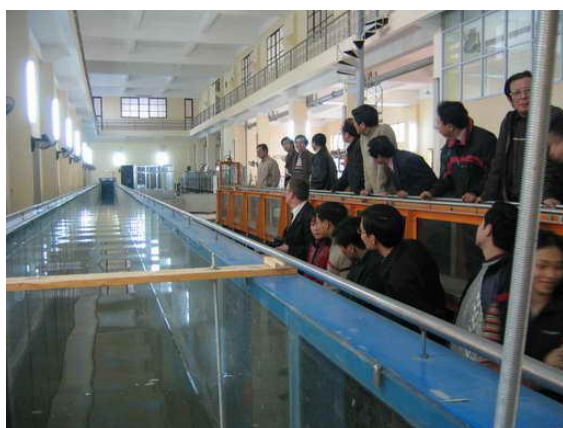
Figure 1: Testing a new wave flume installed in the laboratory, WRU, Hanoi. (photo: WRU - CE)
